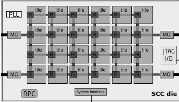
Figure 1. Intel SCC System Overview [5]. A view of the SCC chip showing routers (R), memory controllers (MC) and 24 tiles.
