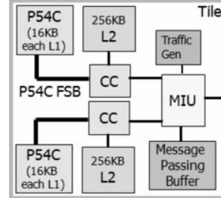
Figure 2. Each of the 24 tiles in the SCC processor contains 2 cores with L1 and L2 caches and a message passing buffer (MPB). The SCC layout and tile architecture showing routers (R), memory controllers (MC), mesh interface units (MIU), cache controllers (CC), and second generation Pentium processor cores (P54C) with their front side bus (FSB) [30].
