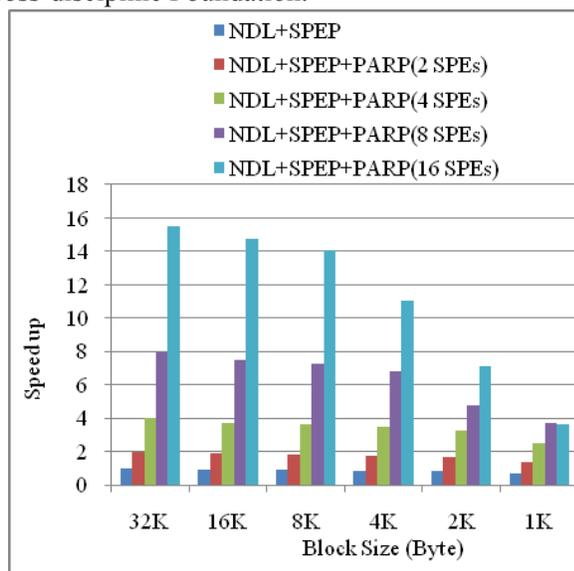
Figure 13. Performance of CellNPDP on the IBM QS20 Cell blade with different sizes of memory blocks and different numbers of SPEs. The baseline is the performance with 32KB memory block size and one SPE. The problem size is 4K. The data are single-precision floating-point.
