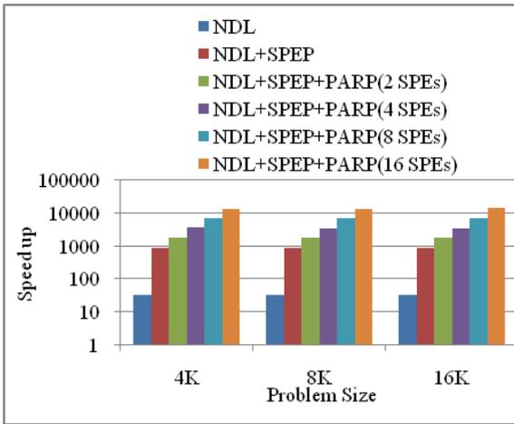
10(a): Speedup on the IBM QS20 Cell blade
