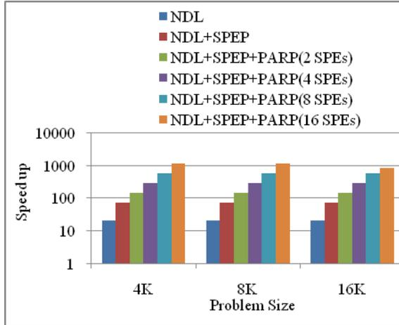
11(a): Speedup on the IBM QS20 Cell blade
