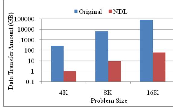
9(b): Data transfer amount on 8-core CPU platform
