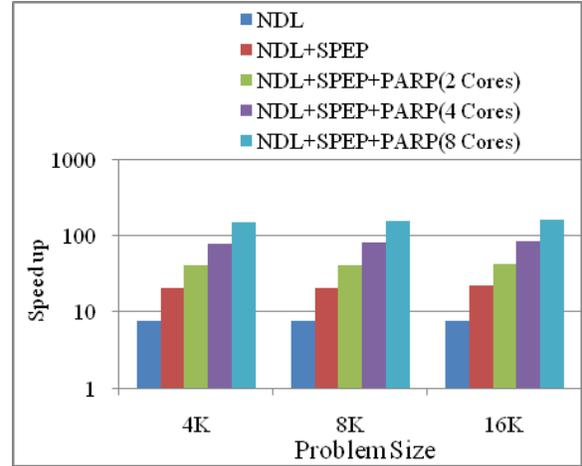
11(b): Speedup on the 8-core CPU platform
