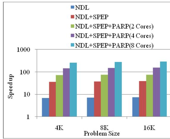
10(b): Speedup on the 8-core CPU platform
