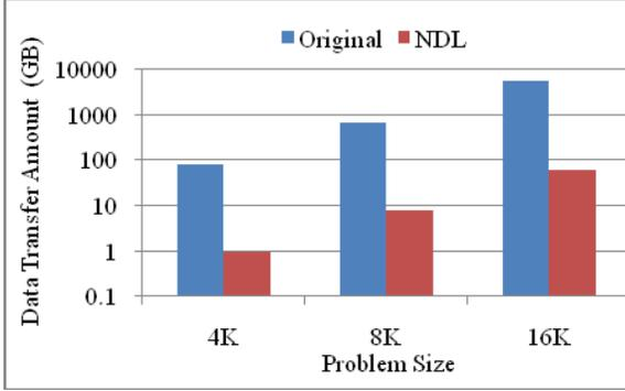
9(a): Data transfer amount on the IBM QS20 Cell blade
