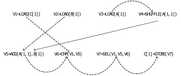
6(b): SIMD instructions of one step for a computing block and the corresponding dependence graph
