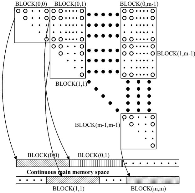
Figure 5. The new data layout of NPDP. Each memory block is a square block whose data are stored sequentially in memory space. Triangular block can be padded into square block.
