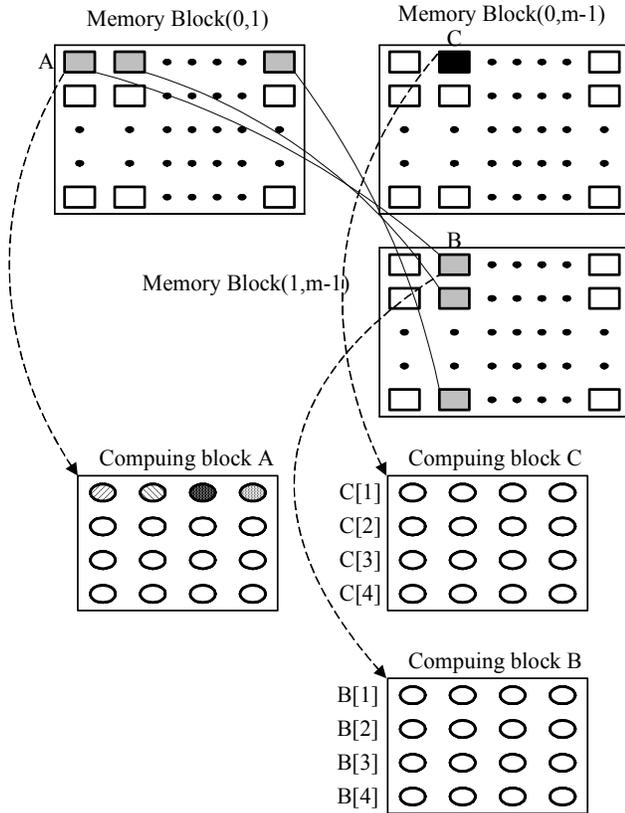
6(a): Memory blocks and computing blocks. The size of each data is 32-bit.
