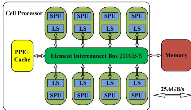
Figure 3. Architecture of the Cell processor
